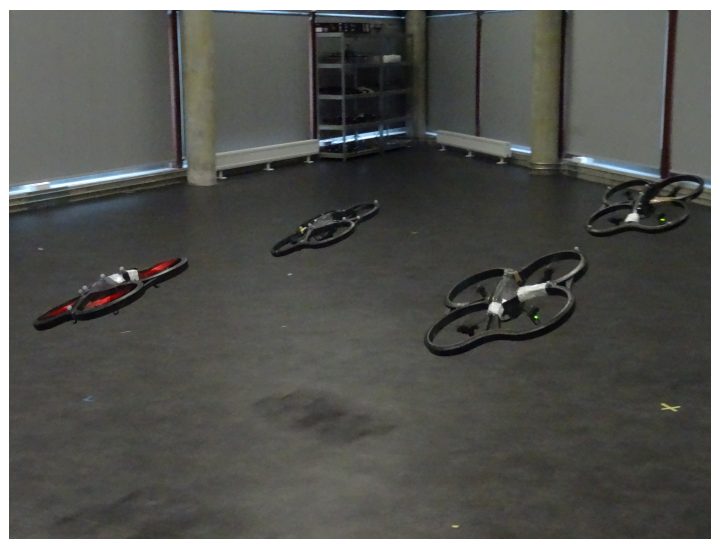
Figure 10. A snap of the real flight of four quadrotors' formation, tracking a circular trajectory while maintaining a rectangle pattern.
