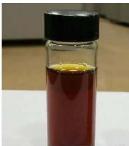
Fig. 2. Graphene oxide produced by Hummer's improved method
