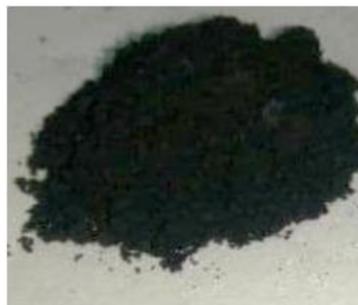
Fig. 3. Shows the reduced Graphene oxide by the thermal method
