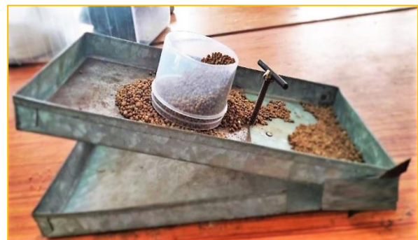
Fig. 4. Measurement the coefficient of friction for granular fertilizers
