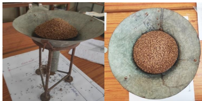
Fig. 2. Measurement the angle of repose for granular fertilizers
