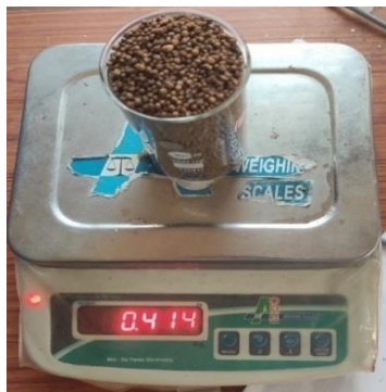
Fig. 3. Measurement the bulk density for granular fertilizers
