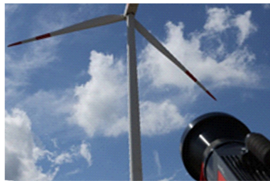
Figure 1. The measurement setup with the IRT camera that aims at the wind turbine from a measuring distance of 190 m.
