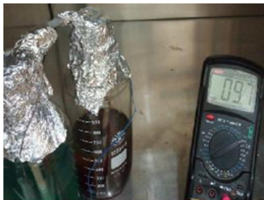
Fig. 7. Current generated using banana peels, mediator and copper as an electrode with S. cerevisiae
