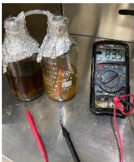
Fig. 8. Current generated using potato peels, mediator and copper as an electrode with S. cerevisiae
