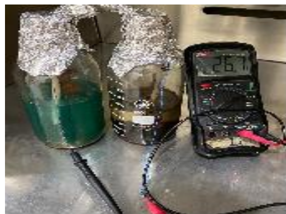
Fig. 4. Current generated using sucrose, mediator and copper as an electrode with S. cerevisiae
