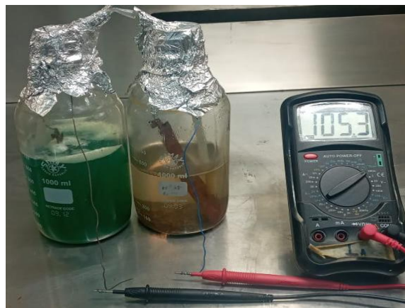
Fig. 3. Current generated using maltose, mediator and copper as an electrode with S. cerevisiae
