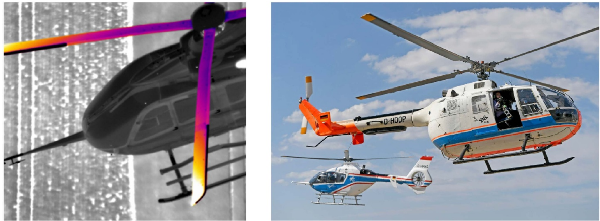
Figure 23. EC 135 in-flight infrared image, blade temperatures highlighted in pseudocolors, with an agricultural field in the background (left), Bo105 chase helicopter with hand-held infrared camera seen in the open passenger compartment (right) [107]
