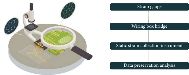
FIGURE 1: Schematic diagram of the site layout of static load test data collection.
