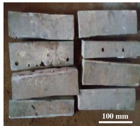
Fig. 1. Aluminum Al-4043 alloy lumps used in the study
