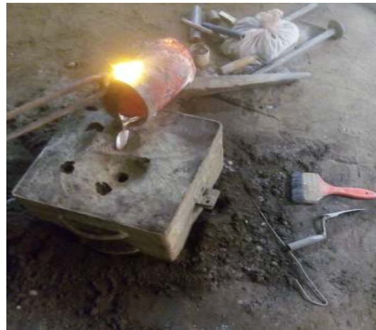
Fig. 3. Cast preparation by pouring the Al/Ni coated SiC slurry from the crucible into the mould
