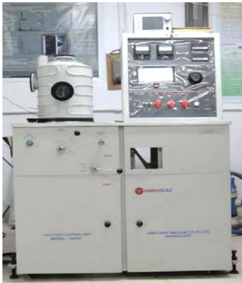
Fig. 2. A model-12A4D vacuum coating machine employed for Ni-coating of SiC particles
