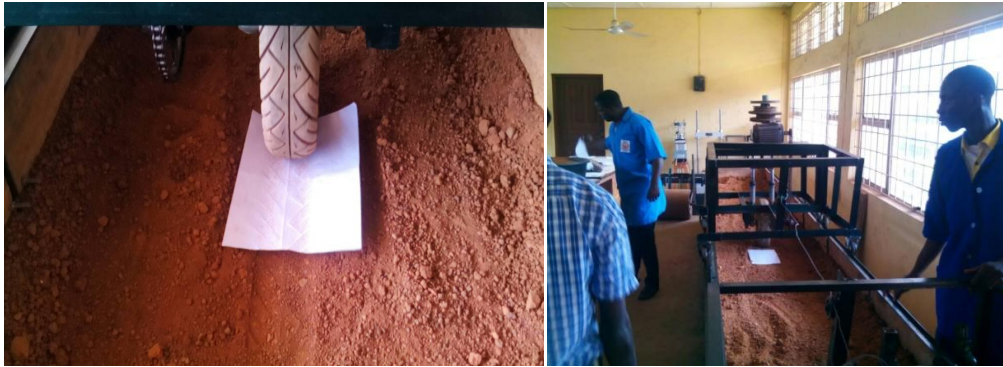
Fig. 5. Testing of the test rig to get the effect of load on the motion resistance and contact area with soil
