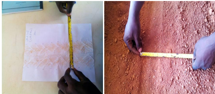
Fig. 6. Measuring the effect of load and inflation pressure on the contact area with soil
