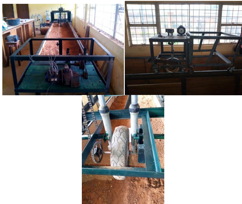
Fig. 3. Drive unit view showing the towing cable, coupling of trolley to the carriage and wheel tester
