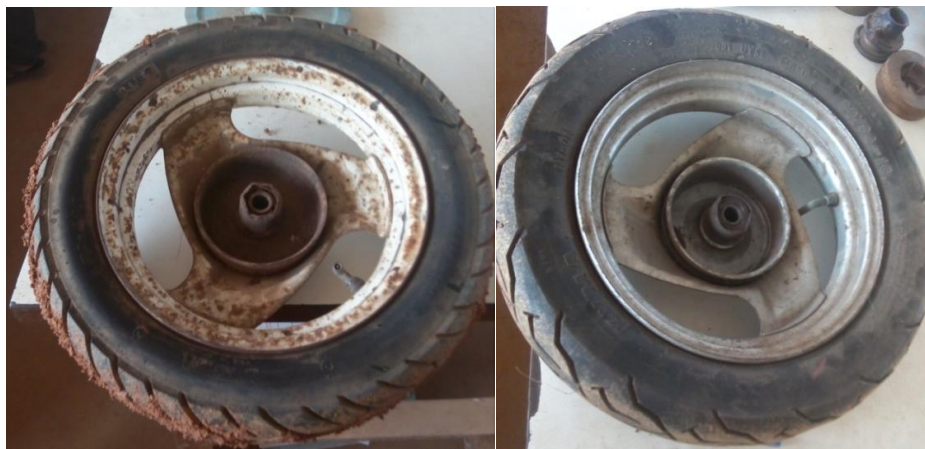
Fig. 4. Test wheel one (1) and test wheel two (2) showing different thread design
