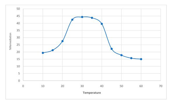
Fig. 4. Effect of temperature on TPH removal efficiency
