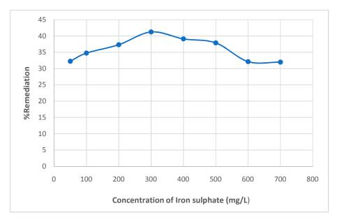
Fig. 2. Effect of  $FeSO_4$  concentration on TPH removal efficiency
