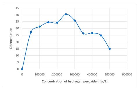
Fig. 1. Effect of H<sub>2</sub>O<sub>2</sub> concentration on TPH removal efficiency
