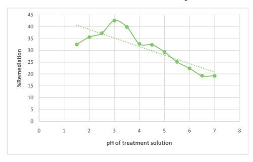
Fig. 3. Effect of pH on TPH removal efficiency
