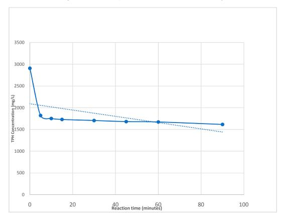
Fig. 5. TPH left after remediation with different reaction time
