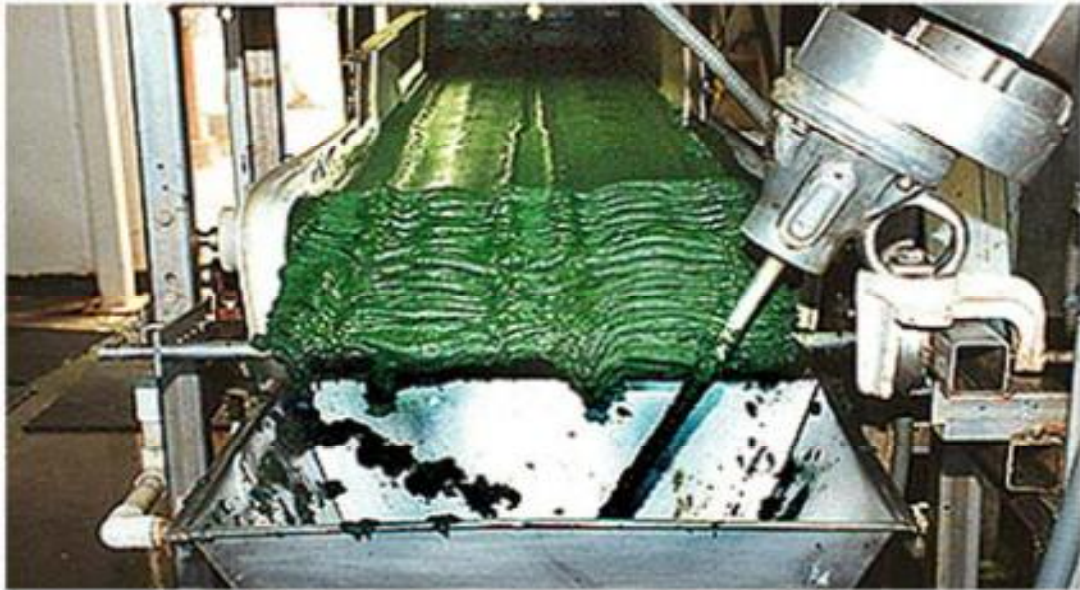
Fig. 3. Microalgal biomass recovered from the culture broth by filtration (Source: [10])
