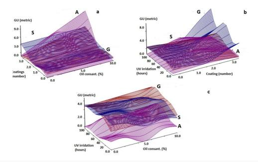
Fig. 4. UV radiations effects on gloss properties of woods (A,G, S: apricot kernel-, grape seedand sesame oil added varnish emulsion; a: coating number and oil concentration, b: UV irradiation time and coating numbers, c: UV irradiation time and oil concentration)
