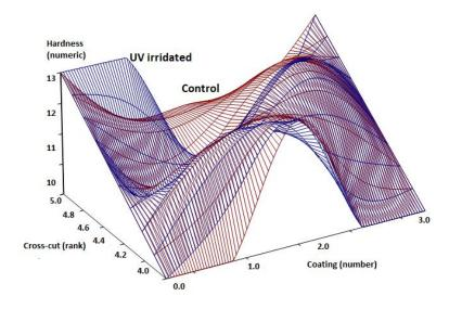
Fig. 3. UV radiations effects on hardness and adhesion properties of woods
