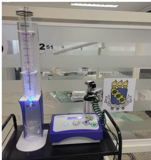
Fig. 2. Ozone generator connected to the hospital oxygen cylinder and the water ozonization tower (Source: O3 Project, 2023)
