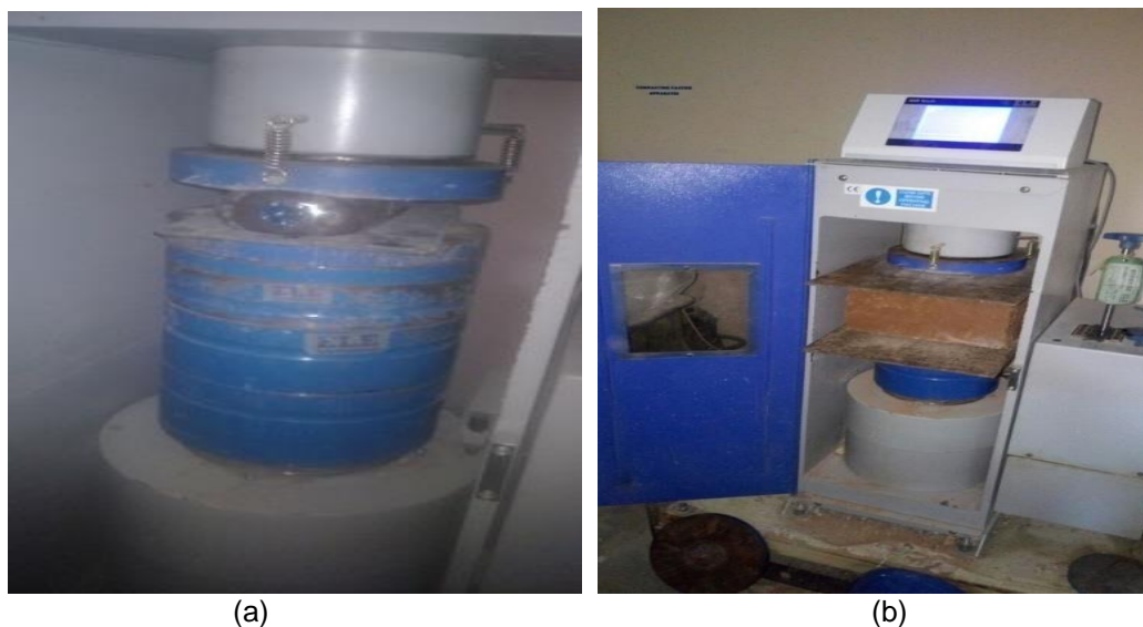
Fig. 2. Compressive strength test (a) empty PET bottle (b) PET brick
