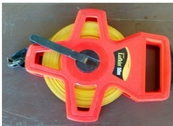
Diameter tape for measuring DBH of larger trees and crown width (CR)
