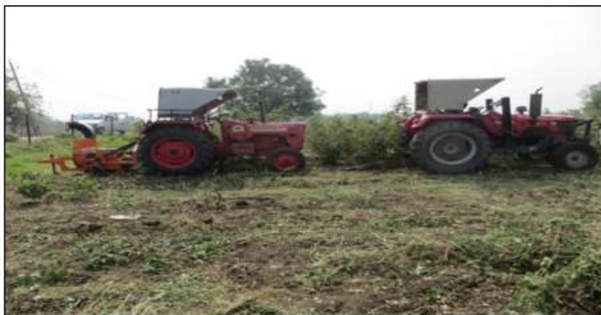
Plate 6. Measurement of draft of cotton stalk shredder cum uprooter using dynamometer
