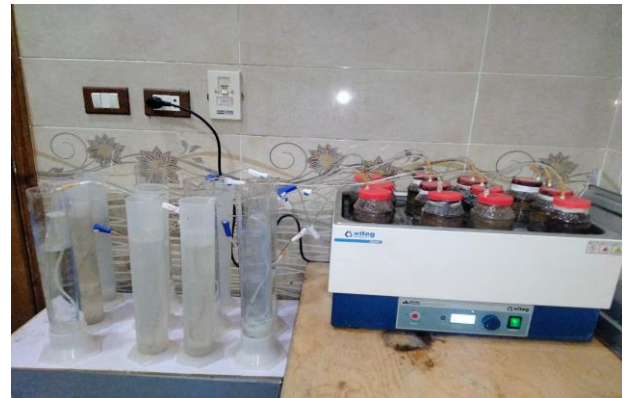
Fig. 4. A laboratory-scale BMP test set-up.
