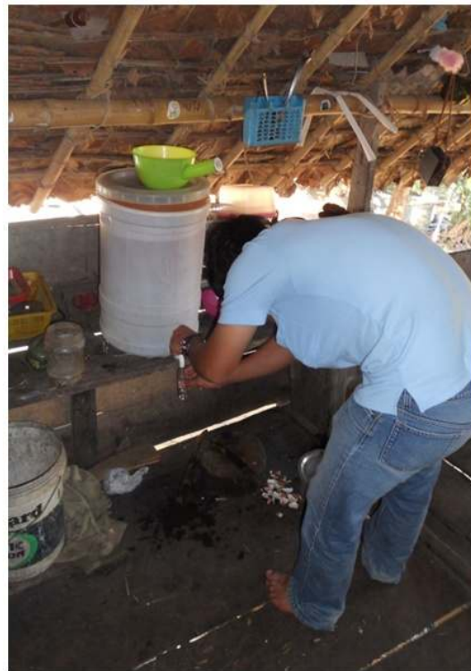
Fig. 4. Sampling the water from the ceramic filter for E. coli analysis
