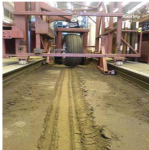
Fig. 1. Off road dynamic facility – soil bin [9]
