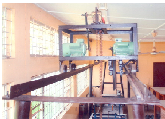
Fig. 8. Indoor soil bin (FUTA) with overhead gantry crane [57]
