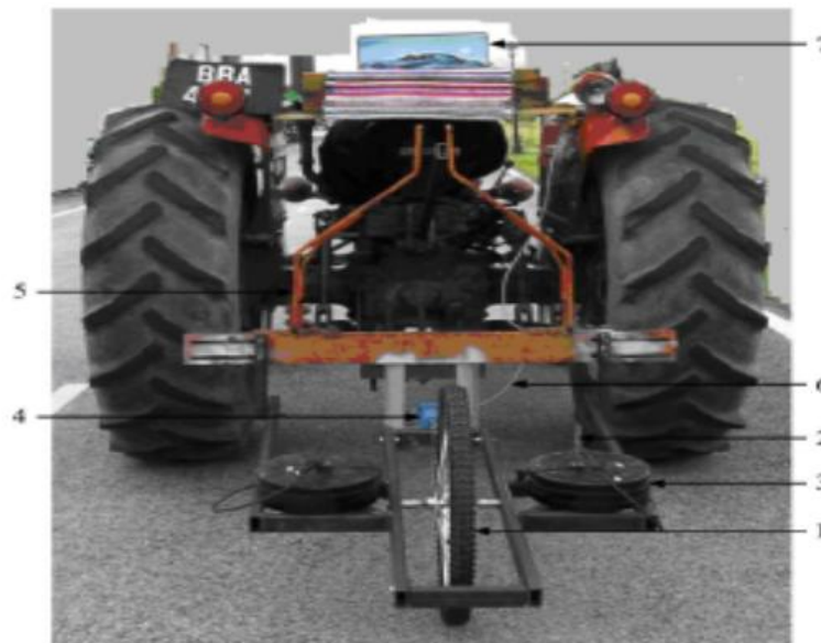
Fig. 4. Test rig coupled to the tractor during field test 1. Test wheel 2. Load hanger 3. Load 4. The BFG 5. Three-point hitch frame 6. Connecting cable 7. Notebook PC [13]
