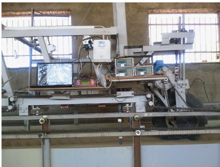
Fig. 5. General view of a single-wheel tester inside soil bin facility [14]
